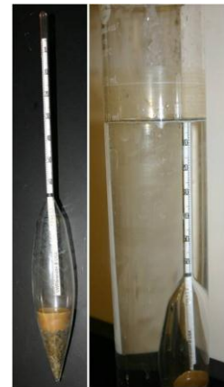
The hydrometer on the left shows the weighted bottom and scale. On the right, the hydrometer floats in water. Note that the water level is at the zero mark on the hydrometer, indicating pure water.
