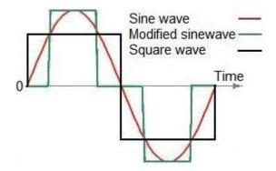
Fig. 4 Sample inverter outputs
