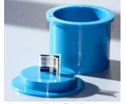
Figure 7: Solar cell with interconnector held perpendicular to the cross section with a UniClip Support Clip before epoxy mounting.
