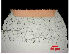
Figure 10: Unetched SAC 305 Solder Alloy.
