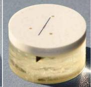
Figure 8: Solar cell interconnects mounted in EpoxiCure® epoxy
