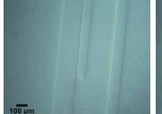
Figure 20: High purity, defect free, polycrystalline silicon viewed with Nomarski DIC (etched with 100mL water, 75g NaOH).
