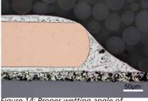
Figure 14: Proper wetting angle of soldered copper
