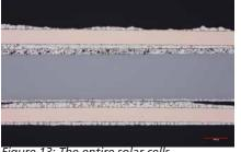
Figure 13: The entire solar cells interconnect shows both the top and bottom soldered seams. The solder is not uniform and lacking at each end of the bottom seam.
