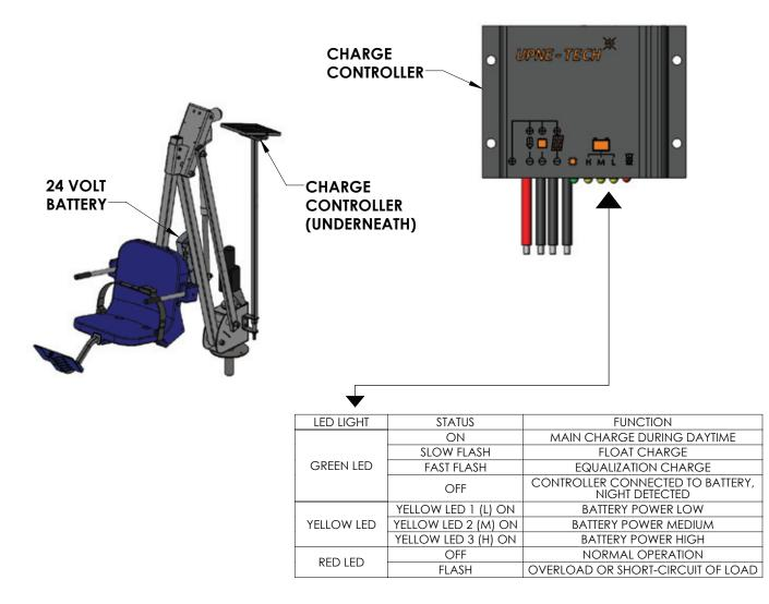
Once the solar charger has been installed and both the control box and battery have been plugged in, and there is sufficient daylight, the 24V Solar Charger will turn on and start trickle-charging the battery. Without both the control box and battery being plugged in, the 24V Solar Charger will be off and will remain off until both components are plugged in.
