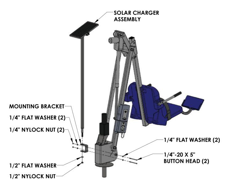
Begin by installing the solar charger assembly to the mounting bracket with the 1/2" flat washer and nylock nut using a 3/4" wrench. Next, intall the mounting bracket to the lift with 1/4" x 5" button heads, 1/4" flat washers and 1/4" nylock nuts using a 1/8" allen wrench and 7/16" wrench.
