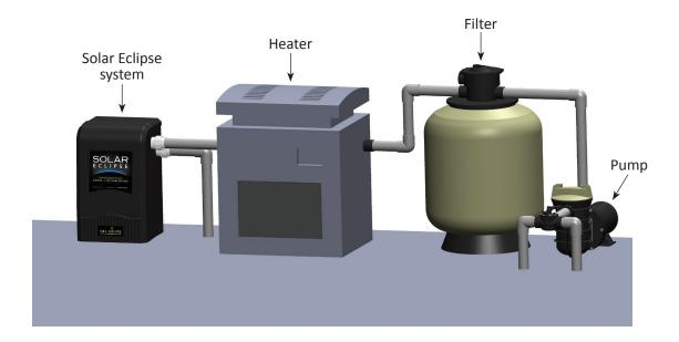
Modern variable speed pumps will work well with Solar Eclipse. The same calibrated spring-driven check valve in DEL's popular standard manifold automatically adjusts for large variations in water flow/water pressure.
