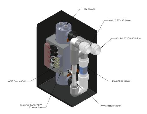
The Solar Eclipse residential pool sanitizer is built primarily from two components – the ozone generator and the UV lamp chamber – which are pre-plumbed and pre-wired. The system installs with simple inlet and outlet unions for water flow and one electrical connection.
