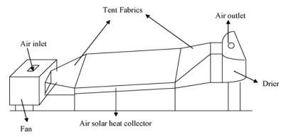
Fig. 10. Rotary column cylindrical drier.
