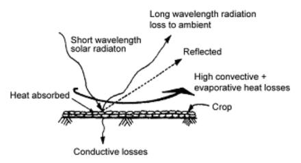
Fig. 1. Working principle of open sun drying.
