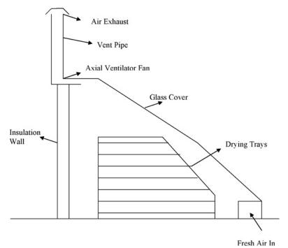
Fig. 6. Green house type solar drier.
