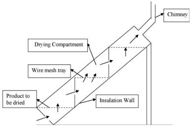
Fig. 9. Staircase solar drier.
