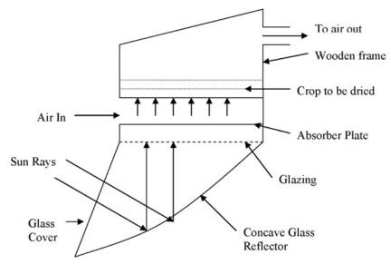
Fig. 4. Reverse absorber cabinet drier.
