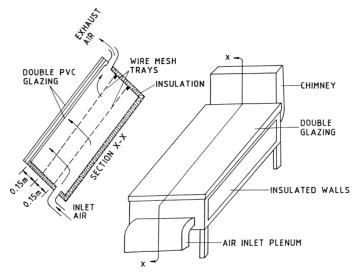
Fig. 3. A modifed natural-circulation solar-energy cabinet dryer.
