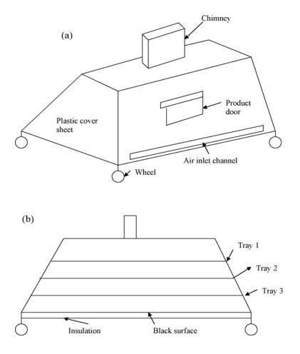
Fig. 13. (a) A simple presentation of first model and (b) side view of first model.
