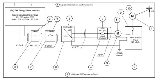
Solar connection details depend on the site and the exact system components. Backfed breaker often needs a 225A busbar, line side connection is easier with a 200A Milbank meter socket. Let's plan ahead together!
