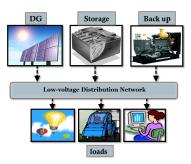
Figure 1. The laboratory-level micro-grid with solar PV panels, battery storage units and lab loads for the UCLA SMERC
