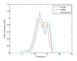
Figure 4. 1 hour-ahead solar generation forecasting and actual data on Jan. 1st, 2011 for the UCLA SMERC
