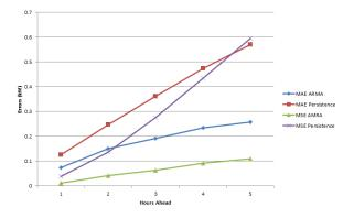
Figure 10. The MAE and MSE of the ARMA model and the persistence model in July, 2011 for different hour-ahead forecasting for the UCLA SMERC
