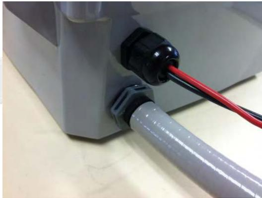
13. Attach the RTU Negative (Black) Wire first followed by the Positive (Red) Wire to the Sun Saver Solar Controller.
