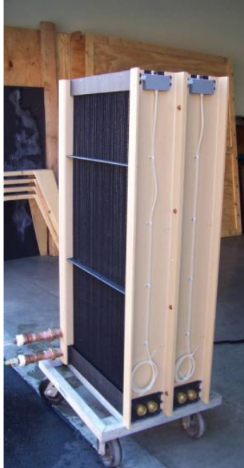
Figure 7. A PPSU regenerator (similar to the one installed in the Tyndall LDAC).
