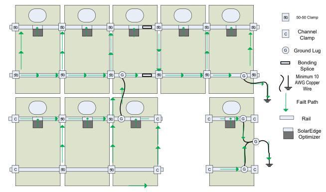
Rail Grounding method with SolarEdge Optimizers
