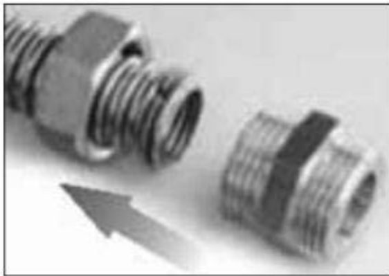
Connect 1" nipple with 1" union nut without flat sealing washer.
