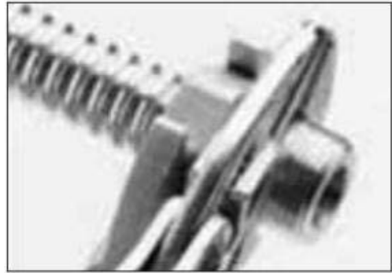
Tighten 1" nipple to 1" union nut, forming a flat-sealing surface.
