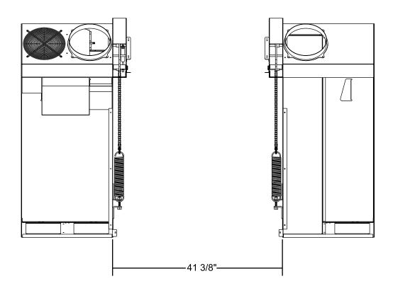
Reattach the bench assembly to the Unscrew the two brackets from the ballast pedestals. Be careful of the wires. Use the drawer and discard. Roll the ballast drawsame screws removed earlier. If needed, er under the bench with the cables toward the hardware kit also contains these 16 the back. screws. The four #10-32 x 1/2" screws hold the back of the bench to the pedestals.
