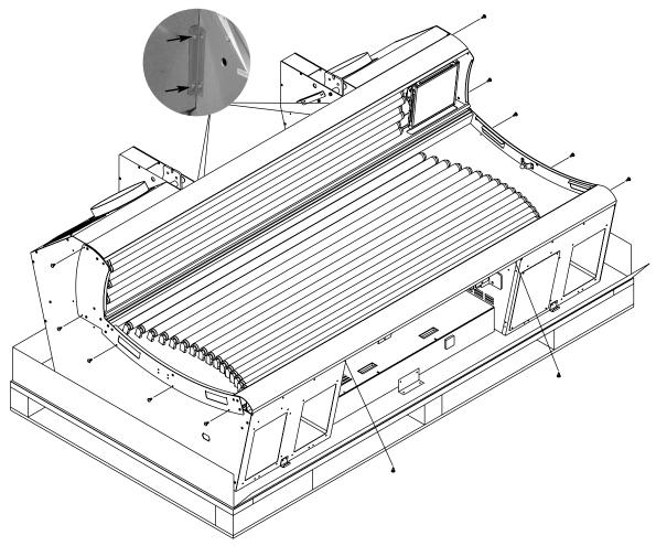
Before lifting the bench assembly, discon- Carefully lift the bench assembly and nect the Shoulder Tanner harness and place upside-down out of the way. blower harness inside the pedestals (see below).
