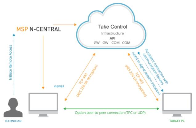
The ports identified in the tables below must be accessible for Take Control and MSP Anywhere remote control connections.
