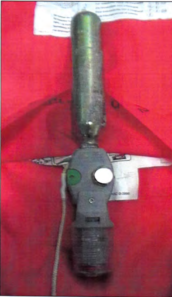
Fig.10. Halkey Roberts inflation mechanism fitted with CO 2 cylinder (as received).
