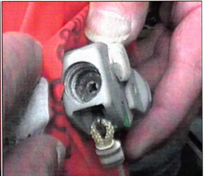
Fig.15. Halkey Roberts inflation mechanism thread – damage at top of thread.
