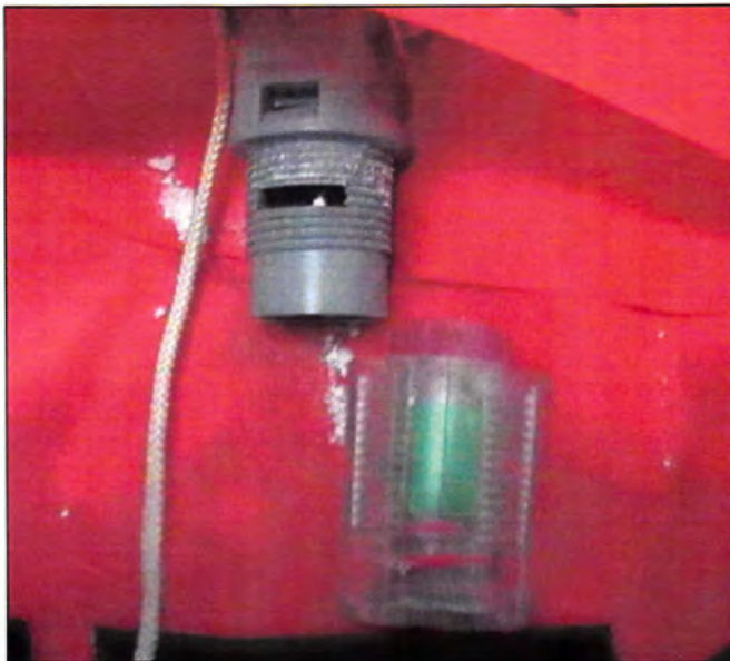
Fig.14. Halkey Roberts inflation mechanism with automatic cap removed.
