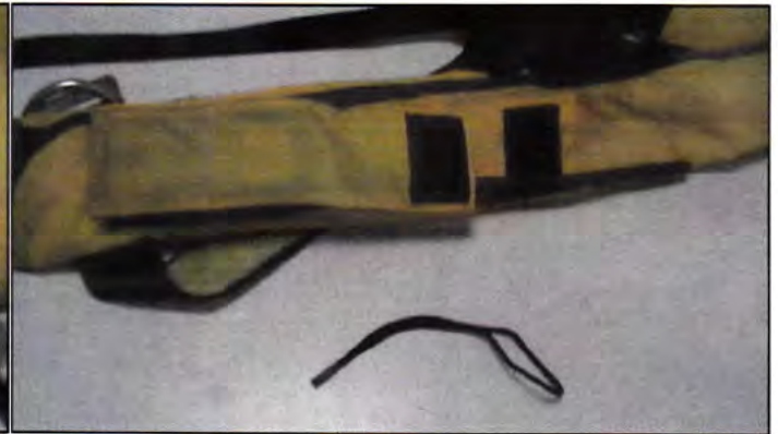
Fig.4. Front pocket with VHF radio and loose cord handle.
