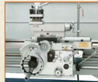
APRON CONTROLS WITH FEED DIRECTION CONTROL
