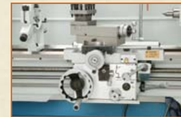
APRON CONTROLS WITH FEED DIRECTION CONTROL
