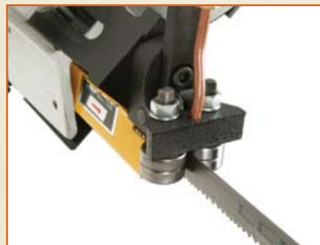
DOUBLE BALL BEARING BLADE GUIDES
