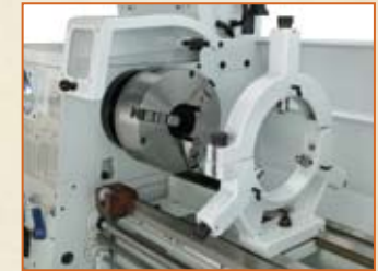
BALL BEARING FINGERS ON EVERY STEADY REST
