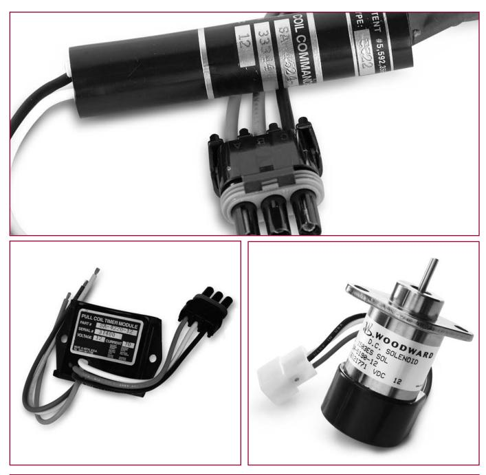
Woodward's extensive line of solenoid protection products feature either external or internal electronics. Coil Commanders<sup>™</sup> and pull coil timer modules (PCTMs) are externally attached to the solenoid to prevent overheating of the pull coil. ICE (Integrated Coil Electronics) and AICE (Advanced ICE) solenoids have built-in electronics that prevent overheating of the pull coil.
