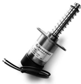
Electronics integrated into a single coil solenoid control the solenoid's current to provide high initial starting force and a constant hold force. The microprocessor encapsulated onto the solenoid calculates the pull time and then generates a pulse width modulated signal to create the hold coil function for single coil solenoids. Under this reduced current, the hold force of the plunger is held constant over input voltage and temperature ranges.
