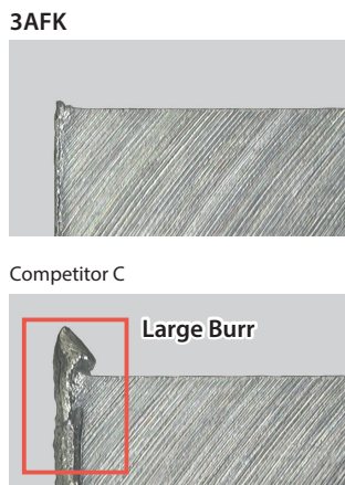
Burr Comparison after Machining (In-house Evaluation)
