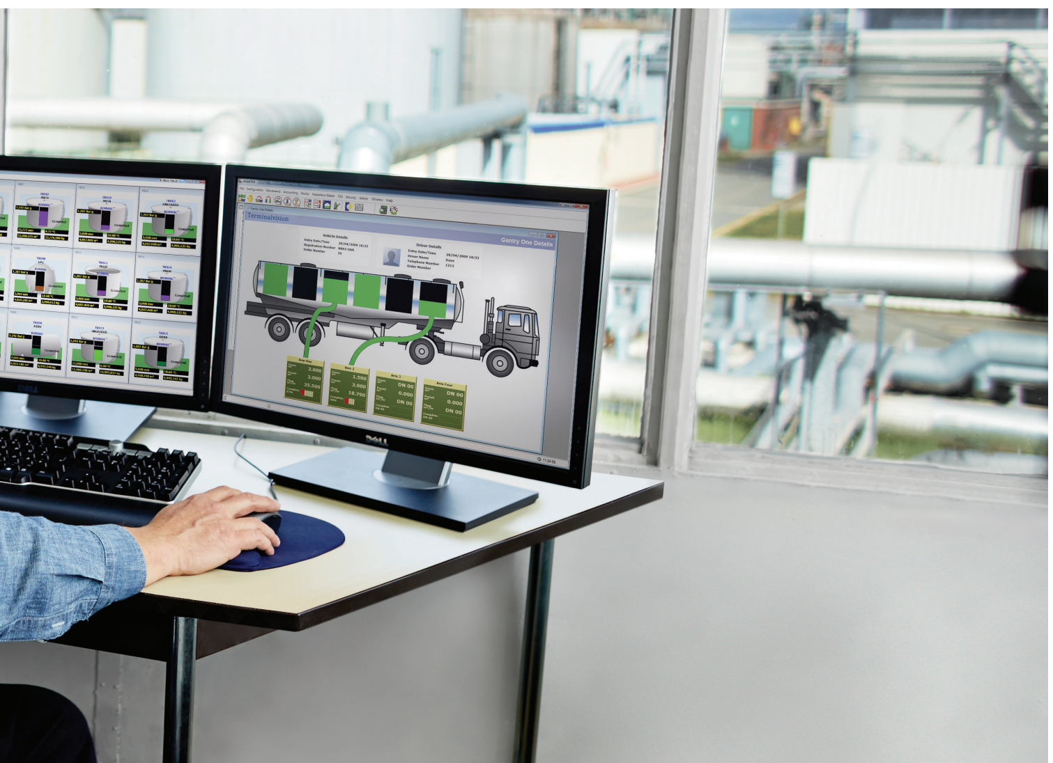
Figure 6: Level data from remote bins and silos can be sent to inventory control software, such as Endress+Hauser's TankVision, which can track inventory worldwide
