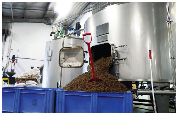
Figure 4: Spent grain is often given to farmers for fertilizer. The brewery needs to monitor level so it knows when to notify farmers for pickup
