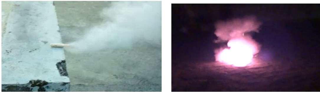
Figure 3: Independent burn test of rocket candy (left), flame temperature test of rocket candy (right).
