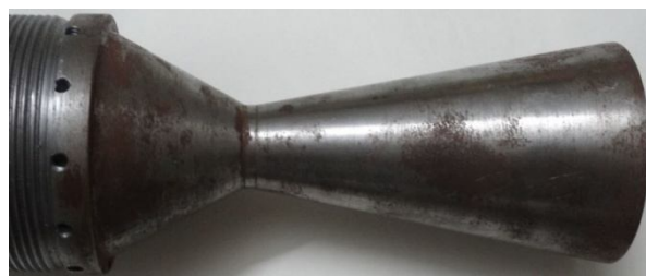
Figure 6: Mild Steel nozzle of prototype rocket motor.
