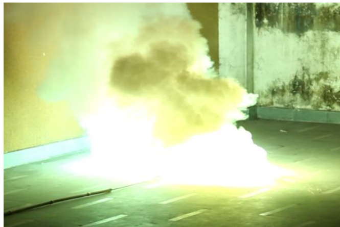
Figure 2: Propellant flame temperature test.
