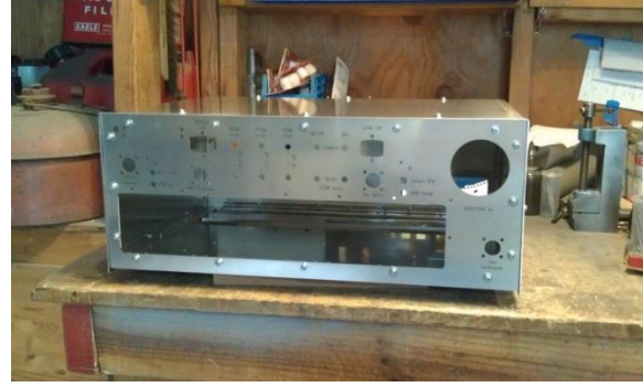
Figure 31: The folded and assembled chassis assembly before painting the top and sides
