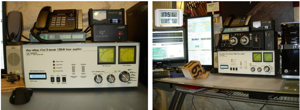
Figure 38: installed in shack. LEFT: idling. RIGHT: “key down” (tongue in cheek, as the photo was taking while transmitting a JT65 cycle), 1.25kW
