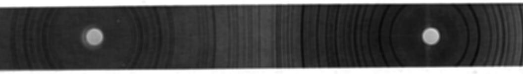
X-ray powder diffraction pattern of  $\mathrm{SiO}_2$  taken with  $\mathbf{Cu}K\alpha$  radiation.
