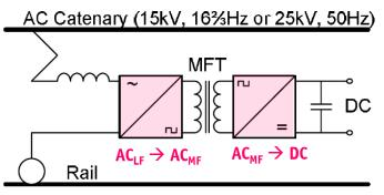
AC-DC conversion with medium frequency transformer (MFT).
