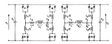
Fig. 5. Double-bridge electronic transformer; arrows define positive polarity of voltages and currents.
