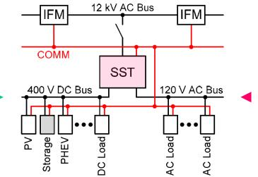
● Bidirectional Flow of Power & Information / High Bandw. Comm. → Distrib. / Local Autonomous Cntrl
