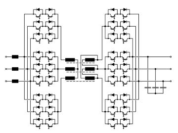
• Example of Three-Phase Integrated (Matrix) Converter & Magn. Phase-Modular Transf.
