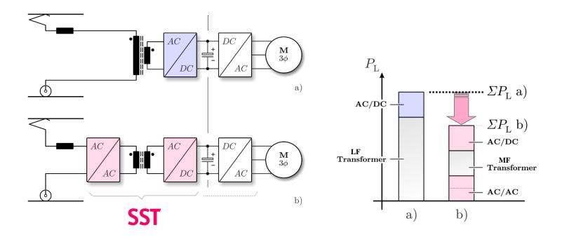
• Medium Frequ. Provides Degree of Freedom  $\rightarrow$  Allows Loss Reduction AND Volume Reduction
