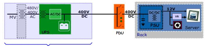
• Future Concept: Unidirectional SST / Direct 6.6kV AC  $\rightarrow$  400V DC Conversion
