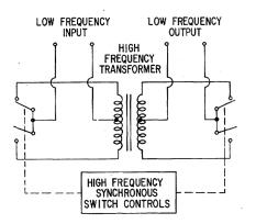
Fig. 1. < Principle of electronic transformer.
