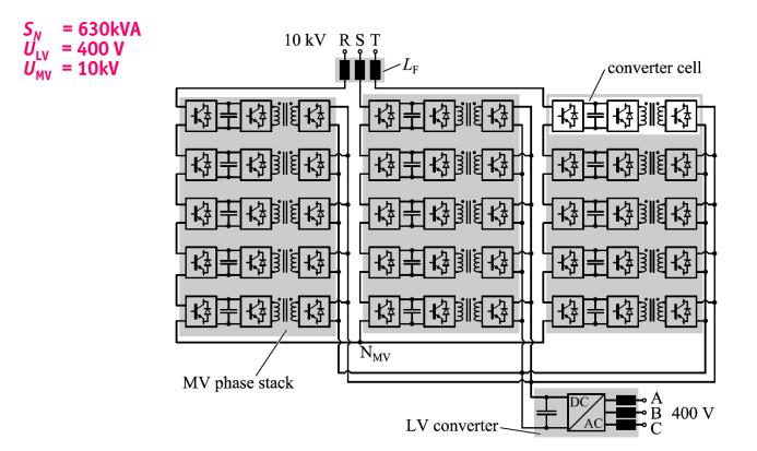
• 2-Level Inverter on LV Side / HC-DCM-SRC DC-DC Conversion / Cascaded H-Bridge MV Structure
