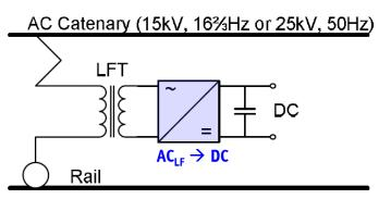
*Conventional AC-DC conversion with a line* frequency transformer (LFT).
