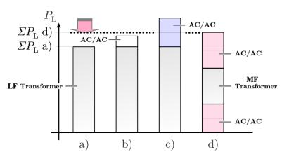
Medium Freq. → Higher Transf. Efficiency Partly Compensates Converter Stage Losses
