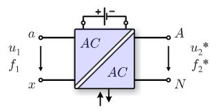
McMurray Brooks EPRI ABB Borojevic Wang etc. Electronic Transformer (1968) Solid-State Transformer (SST, 1980) Intelligent Universal Transformer (IUT<sup>™</sup>) Power Electronics Transformer (PET) Energy Control Center (ECC) Energy Router
