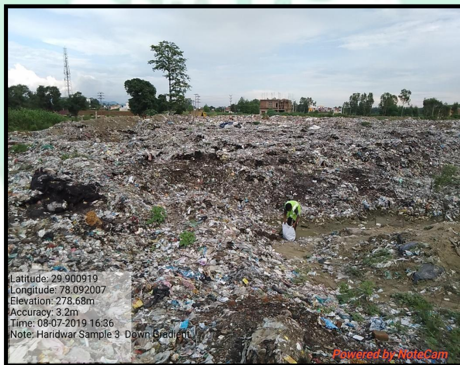
Figure 7: Photo plate Showing Collection of solid waste from Down-gradient (2 meter depth) at location 3.
