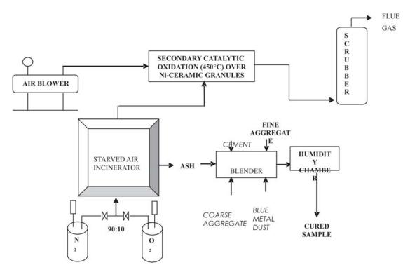
Fig. 1. Schematic Diagram of Starved Air Incineration Followed by S/S Process
