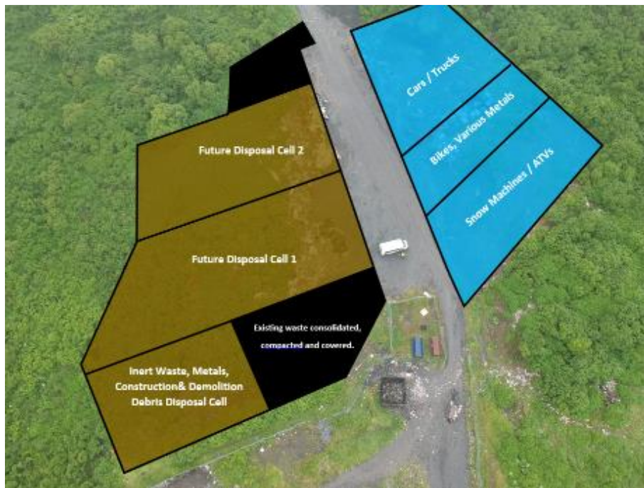
Site plan made from an aerial drone photo. The site plan shows where waste is currently placed, the metals areas, and future disposal cells.
