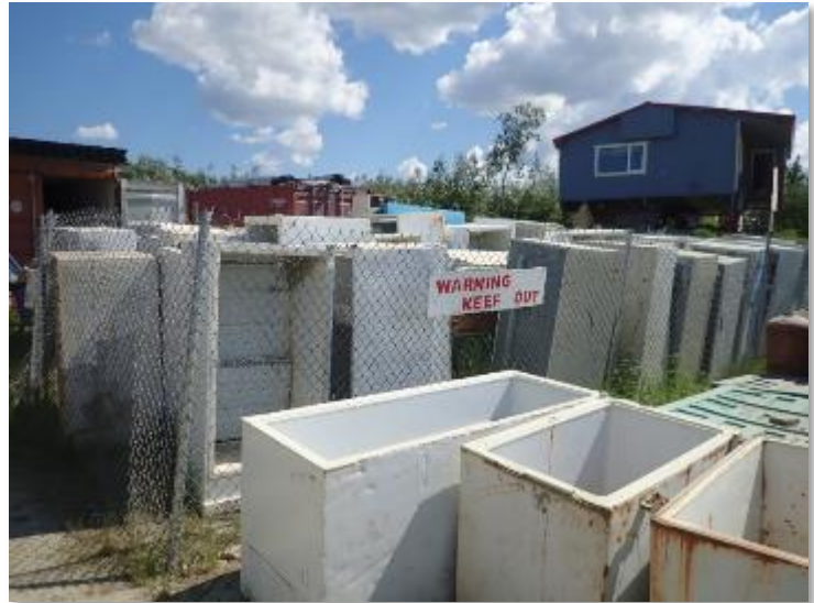
Freezers with the doors removed. To keep them from filling with water they should be stored open side down or in a covered area.
