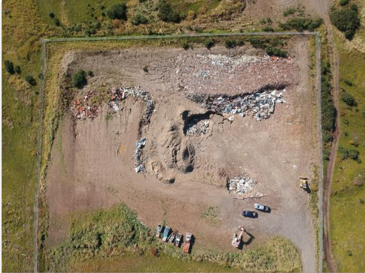
Area fill landfill with two separate working faces demonstrating excellent consolidation. The household garbage working face is near where the cars are parked, allowing easy drop off by the public. The larger working face towards the back of the landfill is for metals.
