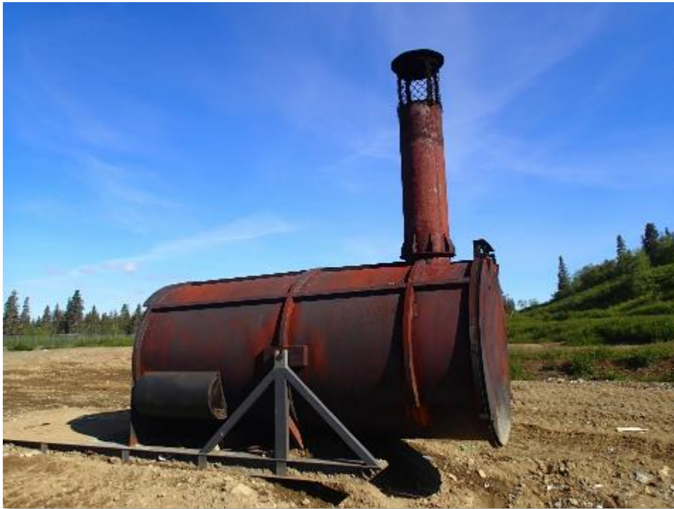
Enclosed commercial burn unit.
