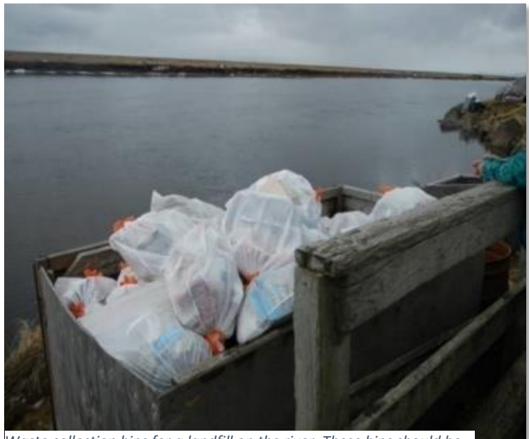
Waste collection bins for a landfill on the river. These bins should be covered to prevent litter and water infiltration.
