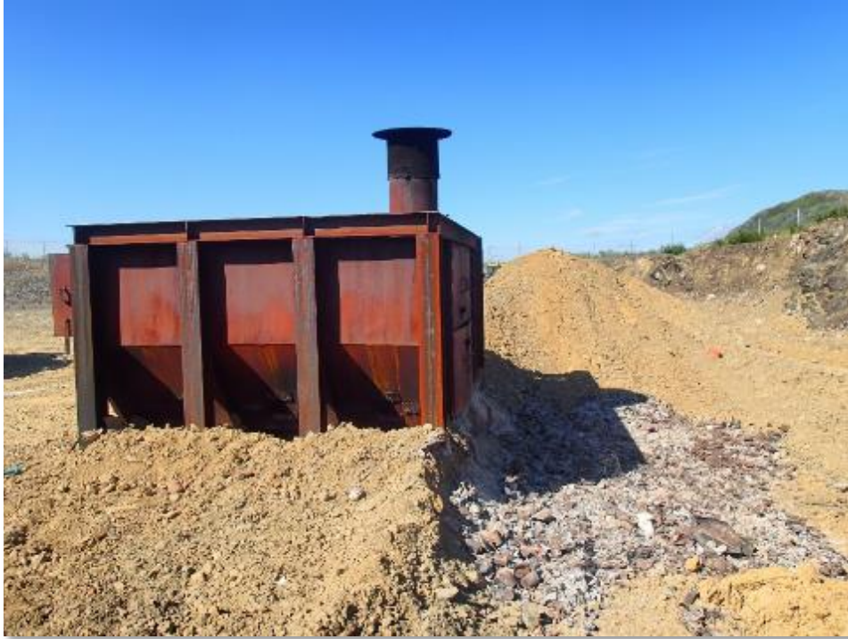
Enclosed commercial burn unit.
