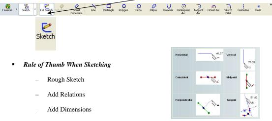
Relations such as parallel, horizontal, vertical and tangent and so on, can be automatically added to the sketch while sketching.
