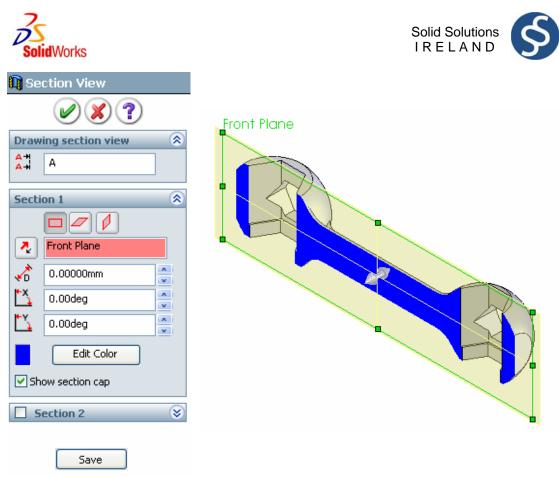
Fig 1.3: Section View and PropertyManager
