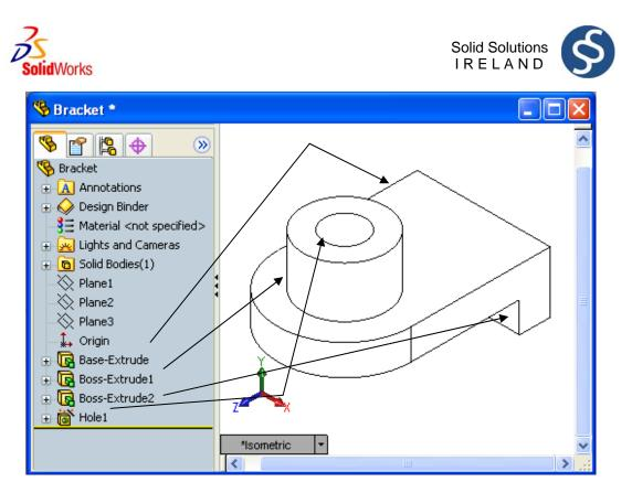
Fig 2.0: Features mapped from their position in the FeatureManager design tree to their position in the model seen in the graphics window
