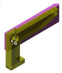
12 Add the Connecting-Rod to the assembly. Use the same SmartMate technique you used in steps 9 and 10 to mate one end of the Connecting-Rod to the end of the Collar.
