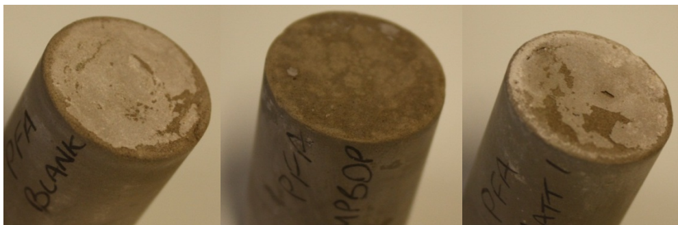
Figure 12: Deterioration of the PFA-series samples. Blank (left), MPBDP (centre) and LUSP 1 (right)
