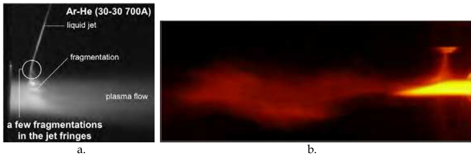
Fig. 5. (a) Example of fragmentation of an ethanol jet, about 300 \mu\text{m} in diameter, starting in the fringes of a d.c. plasma jet (Ar-He: 30-30 slm, 700 A, 40 V, Anode-nozzle i.d. 6 mm) Etchart-Salas et al (2007) , (b) Interaction of an Ar-H 2 plasma jet with atomized ethanol drops Fazilleau et al (2006) .
