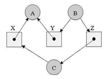
Because there are no cycles in the resource allocation graph, we can see that no process in the system is deadlocked.
