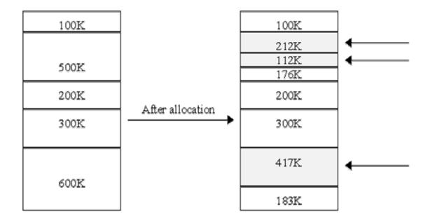
The request of memory allocation for 426K will be rejected, because any single partition in the graph is less than 426K.
