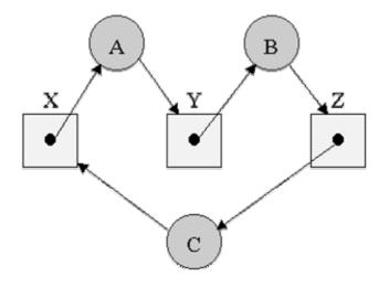
Because each resource type has only one instance, and there is a cycle is the resource allocation graph, we can see that a deadlock has occured.
