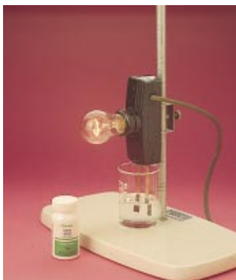
Figure 4 The bulb in this conductivity apparatus lights up if the solute is an electrolyte.
