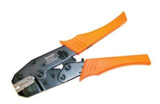
Just center the terminal in the opening of the tool, and give the handle a firm squeeze. You've got a perfect crimp that provides a good, solid connection. When installing a terminal on the igniter, always slide it on straight. Never slide the terminal at an angle or wiggle it from side to side. If you do this, you could cause the terminal to spread and make poor contact. Order additional crimping tools through normal parts ordering channels.
