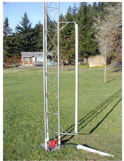
Figure 2, view of the shunt loop at the base of the test tower (28' of Rohn 25G).
