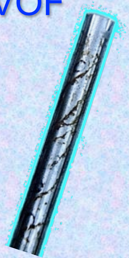
Hydraulic shaft plated with 0.0004" hard chromium after 6 hours of salt spray exposure
