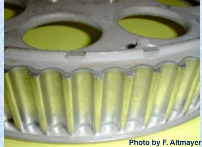
Hard Chromium on Motorcycle Drive Gear
