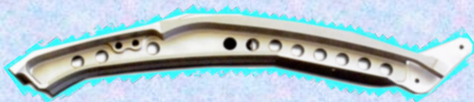
MD-80 Slat Track HVOF sprayed on wear surfaces
