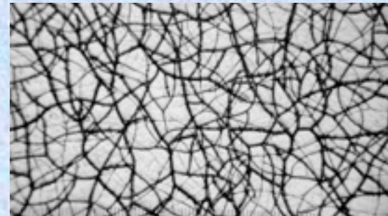
Etched surface of conventional deposit 100X
