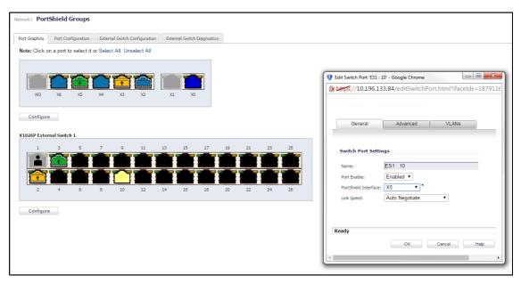
4 Use the VLANs tab to configure an extended switch port in trunk or access mode. In this example, Port 10 is portshielded to X5 and configured as a trunk to carry VLAN 100 by selecting Enabled for the VLAN Trunk option and choosing VLAN 100 from the available list of VLANs:
