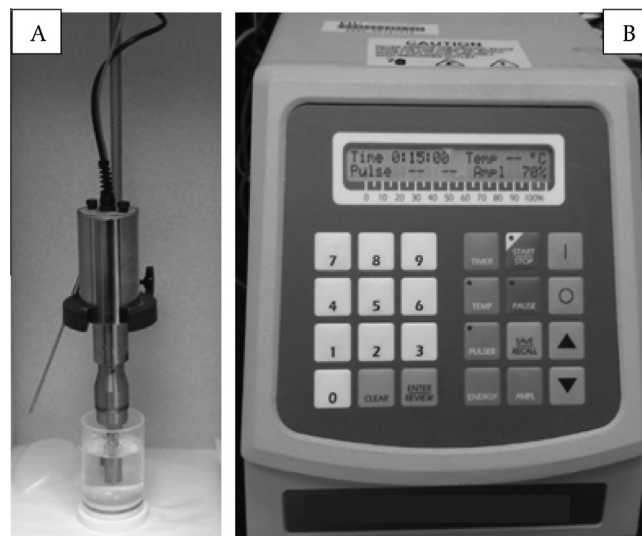
Fig. 5. A simple sonochemical setup for nanomaterial synthesis.
