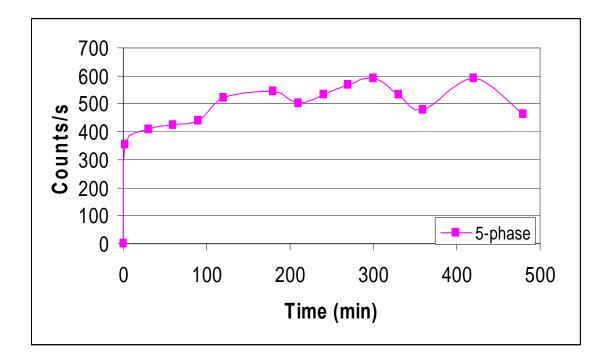
Figure 18. X-ray peak height for 5-phase ( $2\theta$ = 11.9°) as a function of setting time.
