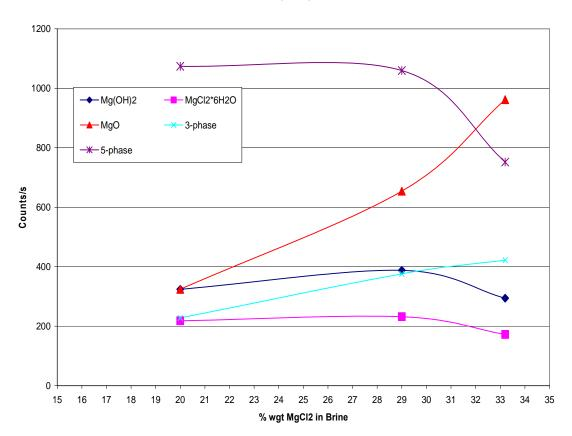
Figure 15. 24 hour x-ray diffraction peak heights from Figure 14 versus "impure" MgCl<sub>2</sub> brine concentration from 20 to 33 % MgCl<sub>2</sub> for cements made with 1.3181 kg/L (11 lbs/gal) impure MgO to brine ratio.
