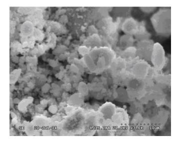
Figure 1. SEM of Premier Chemicals MgO Powder at 3000x Magnification. Dotted Bar = 10 microns.
