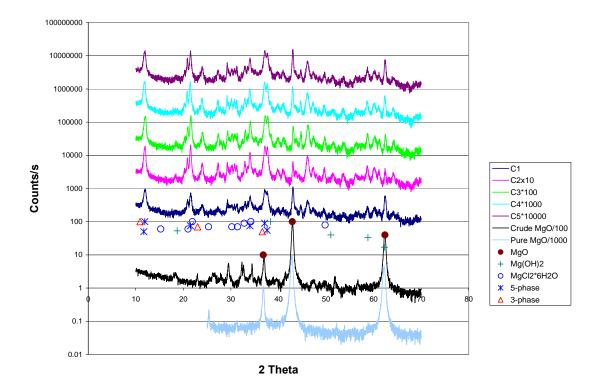
Figure 10. X-ray Diffraction analyses of cements allowed to set for 24 hours. These C series cements were made with various MgO to "pure" 28.9±0.15% MgCl<sub>2</sub> by weight brine ratios given in Table 2. Data points indicate the location and intensity of peaks according to JCPDS-ICDD.
