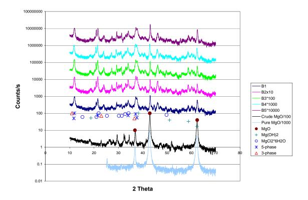
Figure 7. X-ray diffraction analyses of cements allowed to set for 24 hrs. These B series cements were made with various MgO to "impure" 28.9±0.15% MgCl<sub>2</sub> by weight brine ratios given in Table 2. Data points indicate the location and intensity of peaks according to JCPDS-ICDD.
