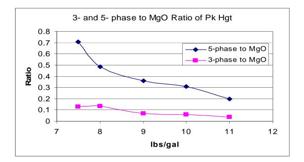
Figure 5. Plot of the ratio of 24-hour x-ray peak heights corresponding to the 5-phase to MgO ratio and the 3-phase to MgO ratio observed in Figure 3 are plotted as a function of the "impure"  $33.2 \pm 0.17\%$  MgCl<sub>2</sub> brine to MgO ratio.
