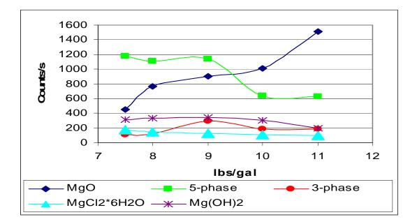
Figure 8. 24 hour x-ray diffraction peak heights from Figure 7 versus MgO to cement ratio for impure 28.9±0.15% weight MgCl<sub>2</sub> Brine and impure MgO.
