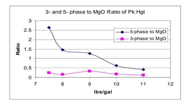
Figure 9. Plot of the ratio of 24 hour x-ray peak heights corresponding to the 5-phase to MgO ratio and the 3-phase to MgO ratio observed in Figure 7 are plotted as a function of the "impure"  $28.9\pm0.15\%$  MgCl<sub>2</sub> brine to MgO ratio.
