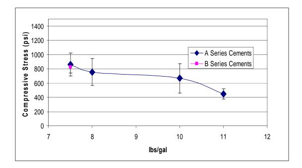
Figure 16. Compressive Strength of Cements as a function of MgO to Brine ratio. These A series cements were made with "impure"  $33.2 \pm 0.17\%$  wgt MgCl<sub>2</sub> by weight brine and the B series cement was made with 'impure"  $28.9\pm0.15\%$  wgt MgCl<sub>2</sub>. Error bars on the data points correspond to the standard deviation of 5 strength measurements.
