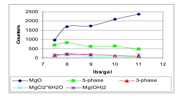
Figure 4. Plot of 24 hour x-ray peak heights corresponding to MgO ( $2\theta$ =42.9°), 3-phase ( $2\theta$ =23°) and 5-phase ( $2\theta$ =11.9°) observed in Figure 3 are plotted as a function of the "impure"  $33.2 \pm 0.17\%$  MgCl<sub>2</sub> brine to MgO ratio.
