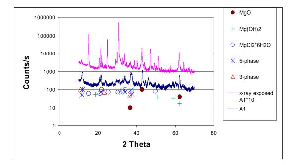
Figure 17. 24 hour x-ray spectra of Cement A1 corresponding to 0.8987 kg "crude" MgO per liter (7.5 lb "crude" MgO per gal) of "impure"  $33.2\pm0.17\%$  MgCl<sub>2</sub> brine when sample is exposed to x-rays for 24 Hrs and when it is not exposed to x-rays.
