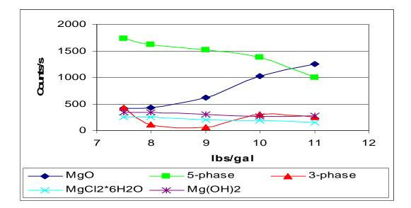
Figure 11. 24 hour x-ray diffraction peak heights from Figure 7 versus MgO to cement ratio for "pure" 28.9±0.15% weight MgCl<sub>2</sub> Brine and impure MgO.
