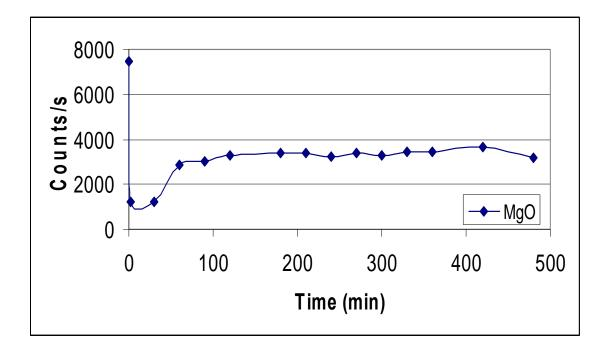
Figure 19. X-ray peak height for MgO phase ( $2\theta$ = 42.9°) as a function of setting time for cement A1 0.8987 kg/L (7.5 lb/gal) 33.2±0.17% "impure" MgCl<sub>2</sub> brine.
