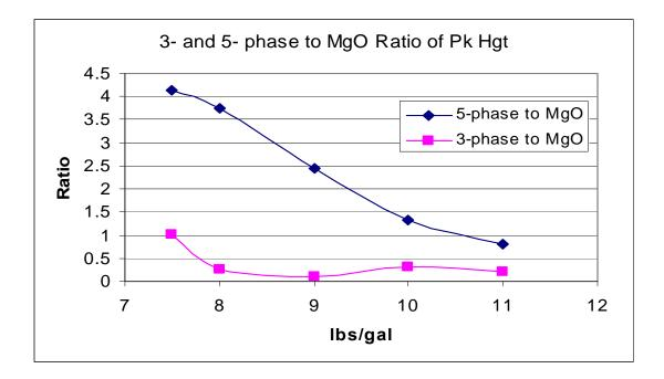
Figure 12. Plot of the ratio of 24 hour x-ray peak heights corresponding to the 5-phase to MgO ratio and the 3-phase to MgO ratio observed in Figure 7 are plotted as a function of the "pure"  $28.9\pm0.15\%$  MgCl<sub>2</sub> brine to MgO ratio.
