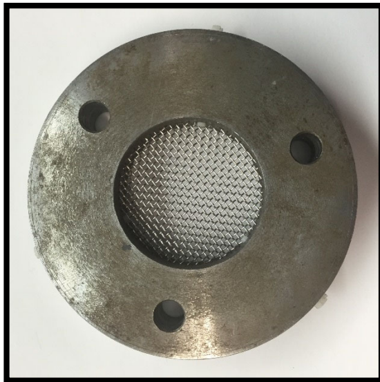
Wire Screen Barrier
