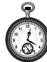
Figure 11.7: Clocks and watches use oscillators to keep time. This works because many oscillators have precisely stable cycles.
