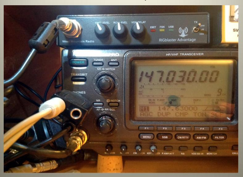
Simple Rigblaster "nomic" only handles sound card TX audio (no mic connection) cost well under \$100
