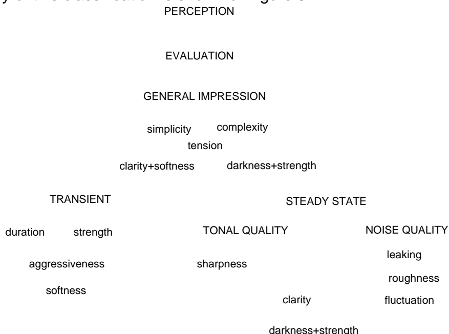
Figure 3. Schematic representation of the structure of attributes found to be suited for a verbal description of flue organ pipe sounds.
