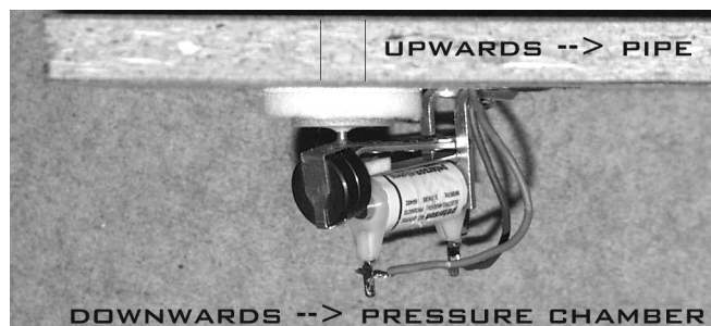
Figure 18. The valve electromagnetically controlled.
