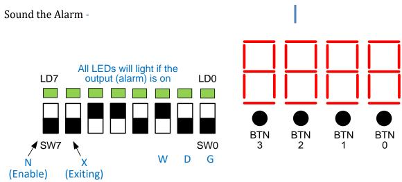
Figure 1 - Switches will be used as the eNable, eXiting, and Windows, Door, Garage sensor inputs. All the LEDs will light up if the Alarm output is 1 (on). The 7-segment displays and buttons will not be used.
