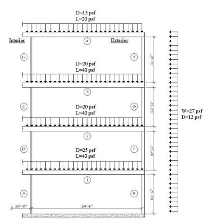
In addition to the loads shown above, 5 psf interior lateral pressure was applied to the studs. For serviceability, a floor joist deflection limit of L/480 for live load was used. Southern Pine was used for the wood studs.
