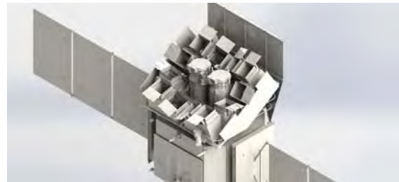
Fig. 5 Layout of the Einstein Probe spacecraft and scientific payloads, which include 12 modules of WXT aligned to different directions and 2 coaligned modules of FXT (credit: MicroSat)
