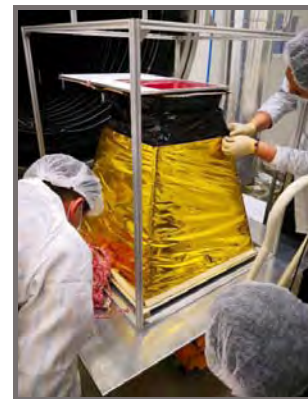
Fig. 6 Preparation for thermal balance test for a WXT module
