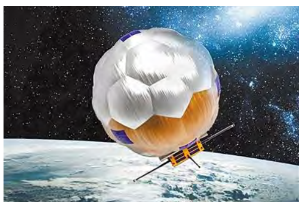
Fig.4 Resistance sail of BP-1B
