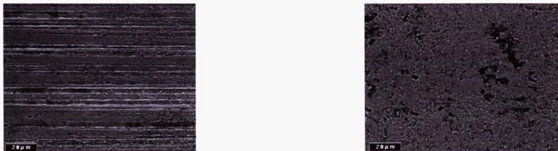
Figure 7. Scanning electron micrograph of the outer raceway in the region above the burnished band (left), and within the burnished band (right)
