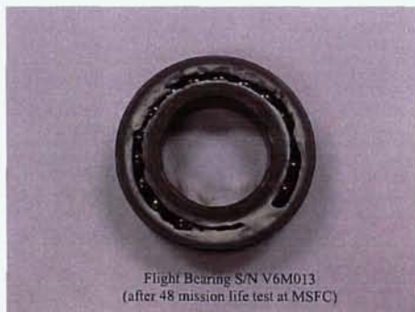
Figure 15. Flight bearing SN V6M013 after 48 mission life test
