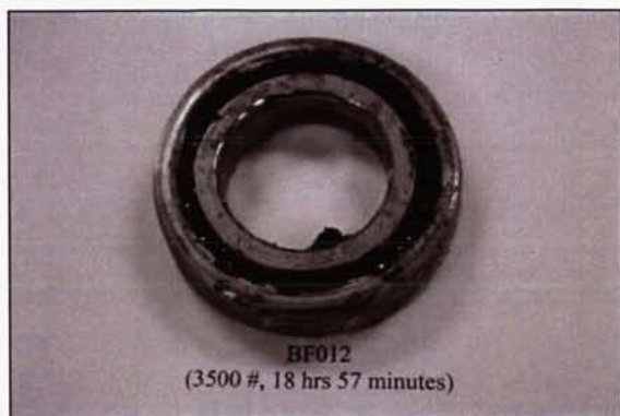
Figure 17. Failed Test Bearing BF012
