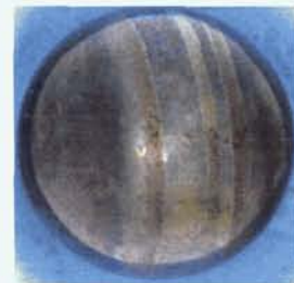
Figure 16. A ball from flight bearing V6L001 after 48 Mission of life tests
