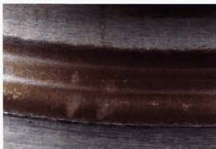
Figure 4. Magnified views of the black wear tracks in the inner race (left) and outer race (right) are shown. Note the false brinelling marks. The dark brown color is an optical aberration of the black color.
