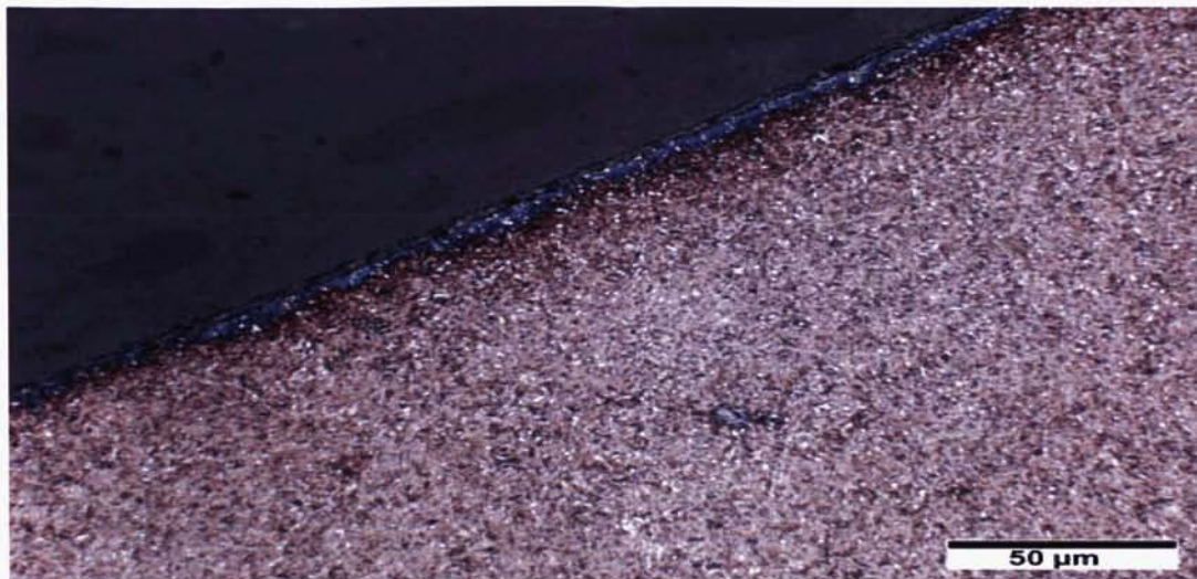
Figure 11b. Metallographic section of black bearing
