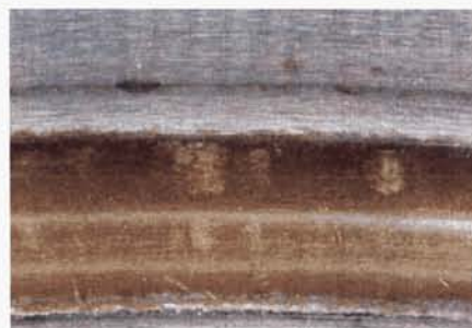
Figure 4. Magnified views of the black wear tracks in the inner race (left) and outer race (right) are shown. Note the false brinelling marks. The dark brown color is an optical aberration of the black color.
