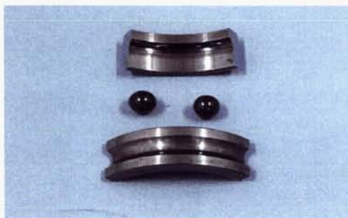
Figure 3. Black bearing after sectioning and cleaning
