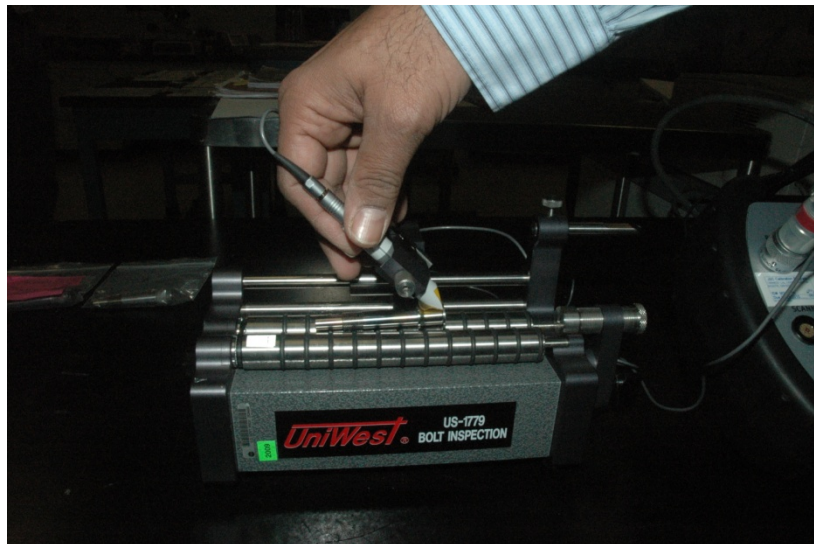
Figure 5.5-1. US 1779 (UniWest) Bolt Inspection Scanner
