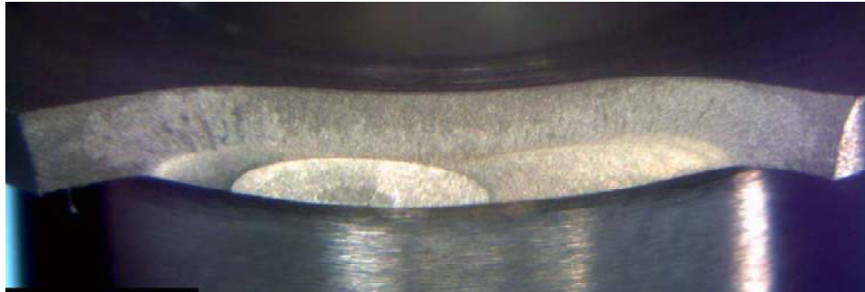
Figure 5.4-10. Image of the Crack Detected in Flight Poppet from STS-126
