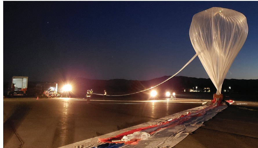
SwRI investigators tested methods for conducting electric and magnetic field measurements of planetary interiors on commercial flights, including the one shown here on a World View Enterprises balloon. These tests helped the SwRI team develop a new instrument that was selected for Artemis. Credit: Earth Science Systems
