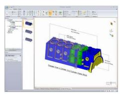
**3D Mark-up** is a documentation environment which includes a set of 3D annotation capabilities and highlighting tools to clearly communicate and document design changes. The environment includes mark-up dimensions, 3D annotations and comparison capabilities. 3D mark-up files can be attached to engineering change requests to clearly and unambiguously communicate the request.
