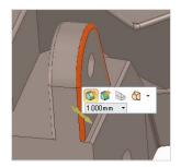
"Heads-up" Display makes use of the latest Microsoft technology, to put relevant commands and choices right where you are working, without getting in the way or requiring you to scroll through drop down menus in search of commands. Fewer mouse movements means more time working with your design.
