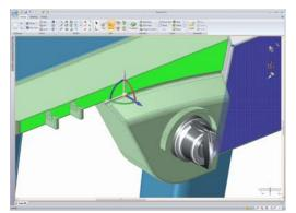
Hints provide helpful, real time feedback to the user as they create or modify geometry. Hints automatically present design considerations, such as maintaining same size holes or wall thickness, in the form of localized "snaps" to similar, surrounding geometry. Hints eliminate the need for the user to enter specific dimensions or interrogate the model before changing or adding geometry.
