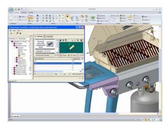
TraceParts Library provides a library of over 100 million standard CAD models from leading parts manufacturers. The library is accessible from within SpaceClaim and the selected component is automatically created and inserted into the assembly.
