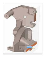
Geometric Inferencing works unobtrusively and in real time to highlight design similarities, such as equal radius holes or coplanar surfaces, during geometry creation and modification, improving user productivity.
