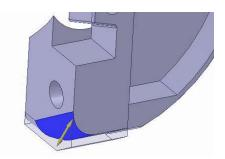
**Pull Tool** creates and modifies geometry with a simple action. Users can pull a surface to create an extrusion, pocket, or hole. Users can also pull a surface to rotate it around an axis or to create sophisticated geometry by blending through different sections. Pulling a profile along a path creates a sweep, and pulling an edge creates a round or chamfer.
