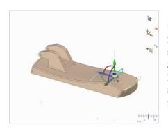
Edit as Blend provides the ultimate in design flexibility by enabling simple geometric shapes, such as a cylindrical surface, to be modified into a blended surface. The tool allows placement of 2D sections throughout the geometry and the ability to modify the 2D sections of any model, regardless of where it originated.
