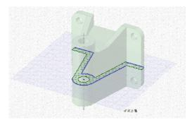
**Section Tool** provides a way to modify a 3D model by directly changing section geometry located at any cross section through the design. This intuitive operation is familiar to those used to working in 2D.
