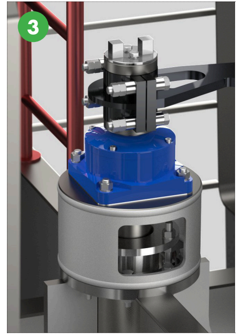
3 The top bearing assembly of a 20 meter windfarm vessel rudderstock
